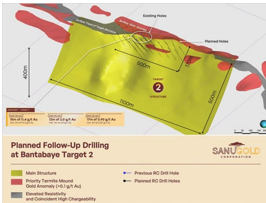
**Figure 2:** Target 2, orthographic view towards the northwest and slight down from above. 3D model of the main structure at Target 2 and Phase 1 follow up drilling, integrating the geophysics, surface data and drilling data. The grey polygon at surface is the surface trend of the key structure mapped by elevated resistivity and coincident high chargeability.
